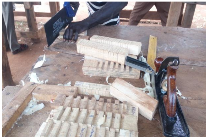
A sample mortise and tenon joint made by the trainees.
