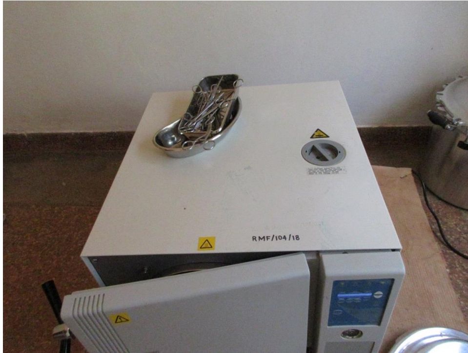
The sterilization machine at Panyadoli Health Centre III. This used to sterilize the equipment in the Operating Theatre to prevent infection.
