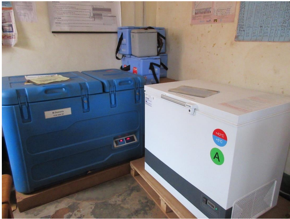
Some of the equipment in the EPI section, which is important for maintaining the temperature of vaccines in order to keep them safe and effective for use on babies.
